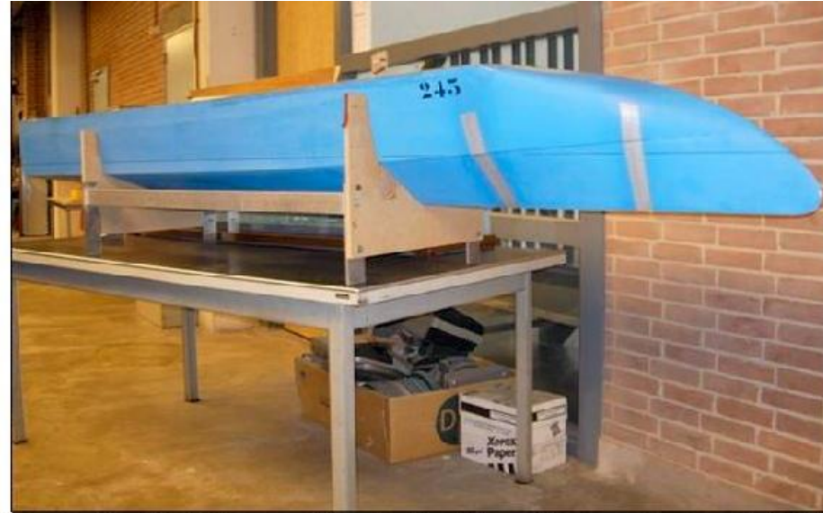
Figure 5b: Model according to the Wave Piercer Concept (WPC)
