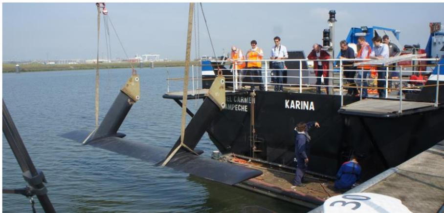
Figure 7. *The installation of the Hull Vane<sup>®</sup> onto the transom of the 55m Supply Vessel Karina.*
