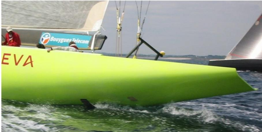
Figure 1. The second application of the Hull Vane<sup>®</sup>, on the 2003 IACC yacht *Le Défi Areva*.
