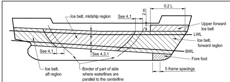
Figure 8 [Ship ice belt regions for 1C FS & 1B FS (FSICR, Section 4.1, Figure 3)]
