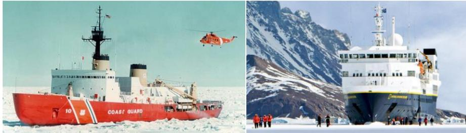
Figure 1 [Left: USCG Polar Sea (PC icebreaker, Cat A), Right: M/V National Geographic Explorer (DNV Ice Class 1A, Cat B)]
