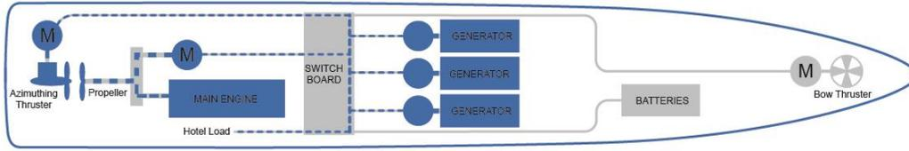
Figure 13: Breathe propulsion High speed mode
