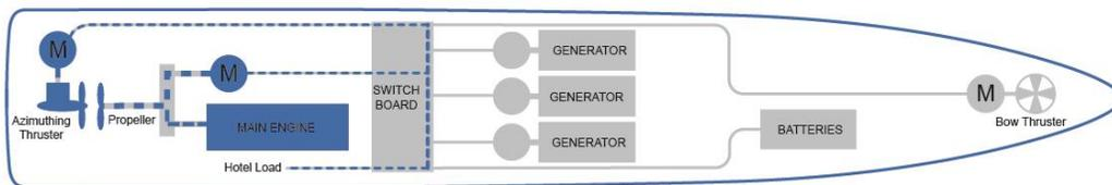
Figure 12: Breathe propulsion Range mode
