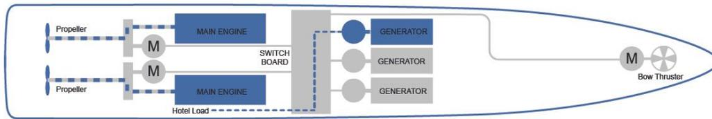
Figure 9: Hybrid propulsion high speed mode
