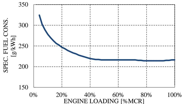
Figure 4: Specific fuel consumption versus engine loading
