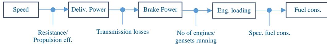
Figure 14 Calculation method for the fuel consumption
