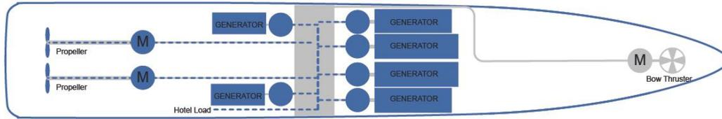
Figure 6: Diesel Electric propulsion
