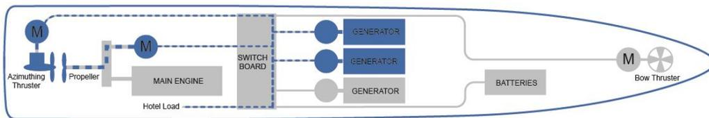
Figure 11: Breathe propulsion Diesel Electric mode
