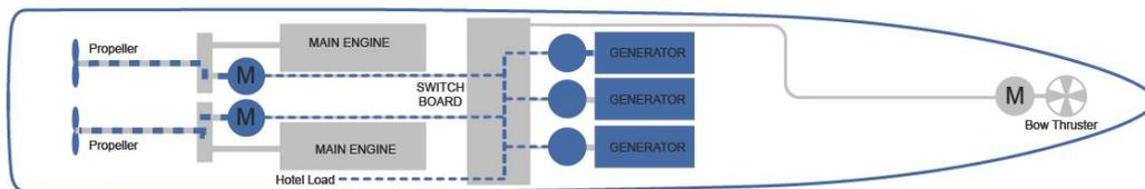
Figure 7: Hybrid propulsion PTI mode
