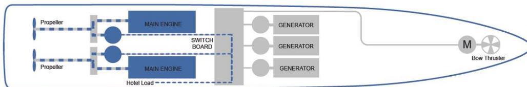
Figure 8: Hybrid propulsion PTO mode
