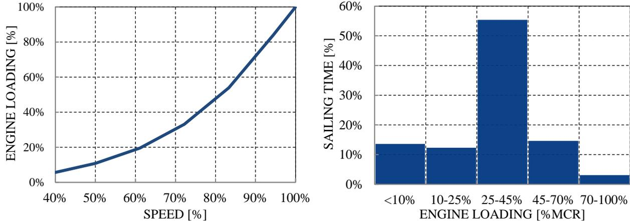
Figure 3: Engine loading versus speed and engine loading distribution
