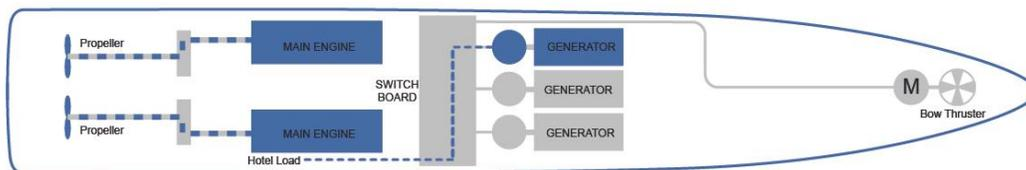
Figure 5: Reference case, conventional propulsion
