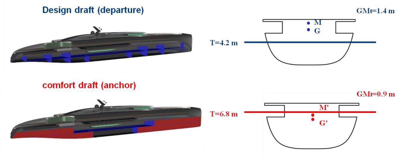
Figure 10: Principle of the comfort draft
