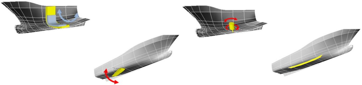
Figure 1: Different types of roll stabilising devices
