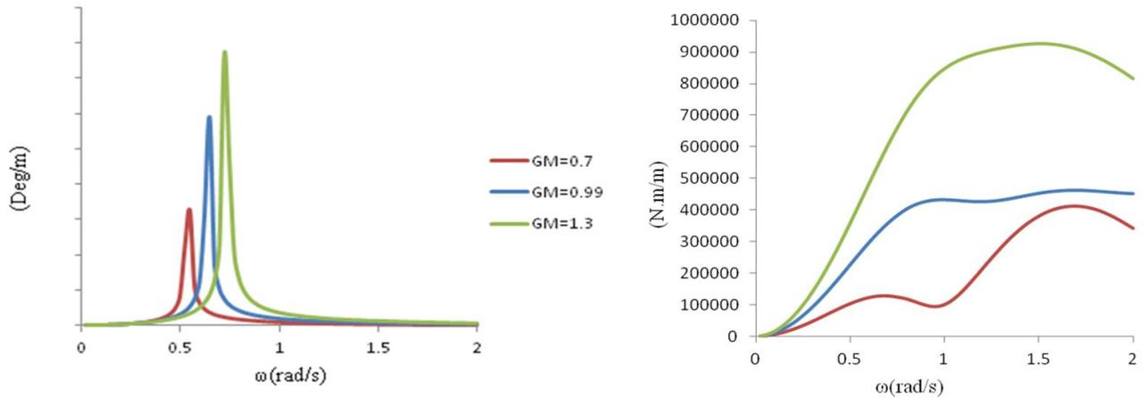
Figure 2: RAO of roll and roll excitation as function of wave frequency
