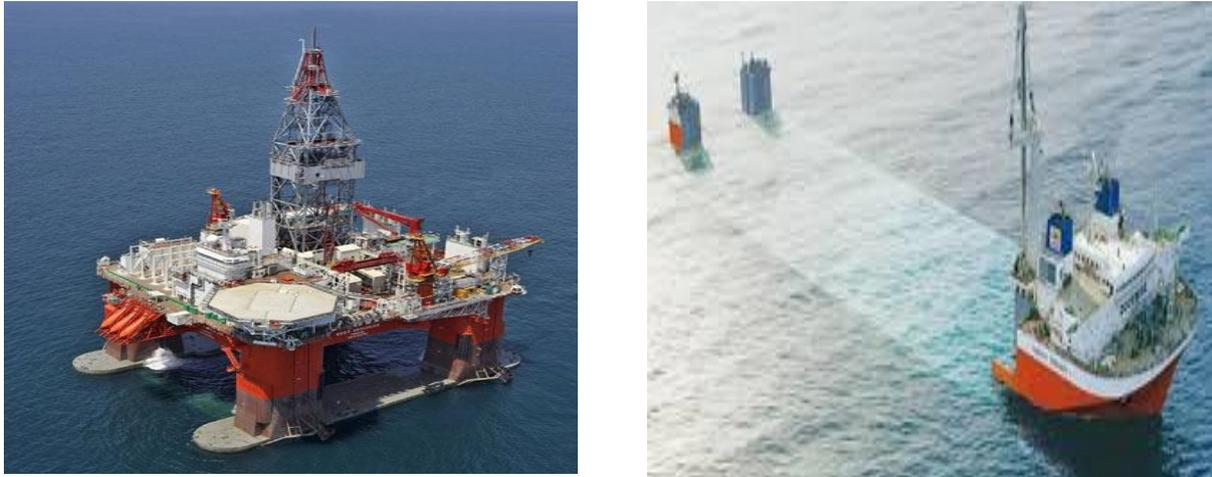
Figure 4: Semi-submersible and submersed heavy transport vessel
