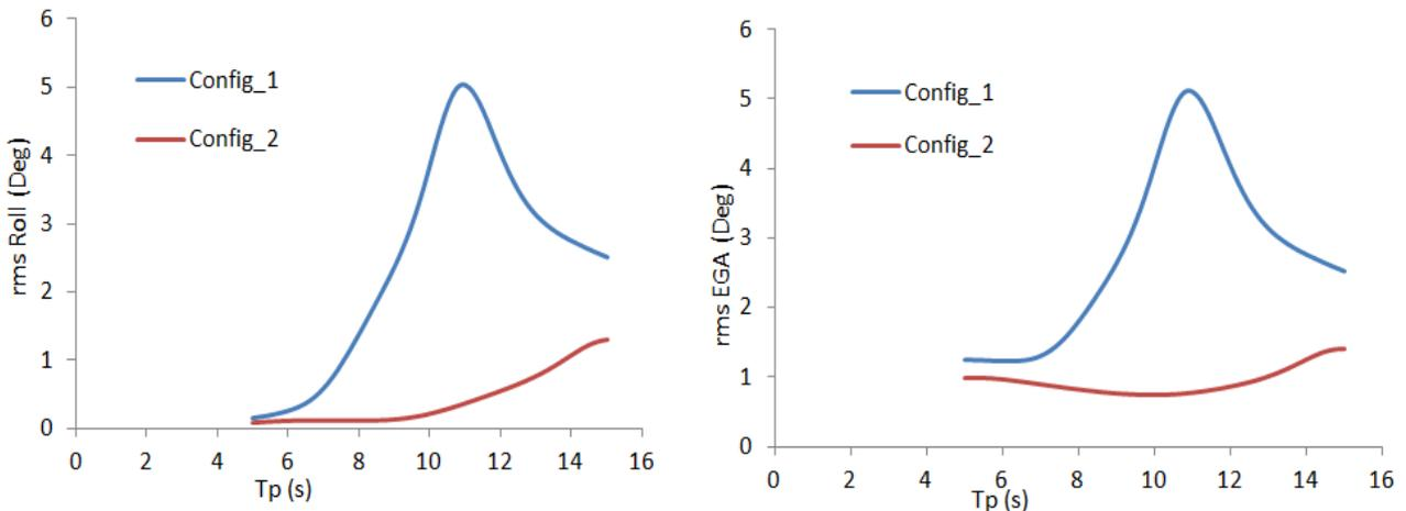
Figure 13: Standard deviation of Roll (left) and EGA (right) for different  $T_p$  and for  $H_s=1m$  in beam seas
