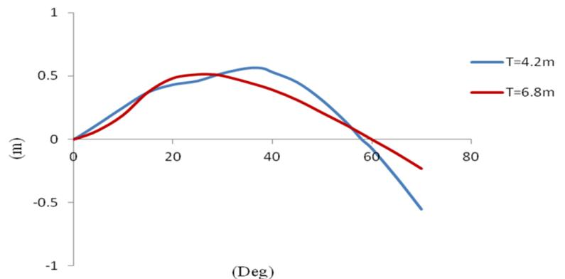
Figure 9: GZ curve and stability criteria
