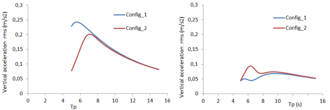
Figure 17: Standard deviation of vertical acceleration in beam seas (left) and bow-quartering seas (right) for different  $T_p$  and for  $H_s=1m$
