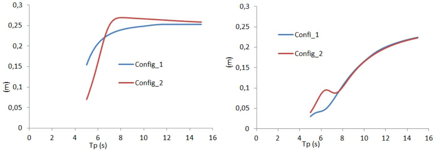
Figure 16: Standard deviation of Heave in beam seas (left) and bow-quartering seas (right) for different  $T_p$  and for  $H_s=1m$
