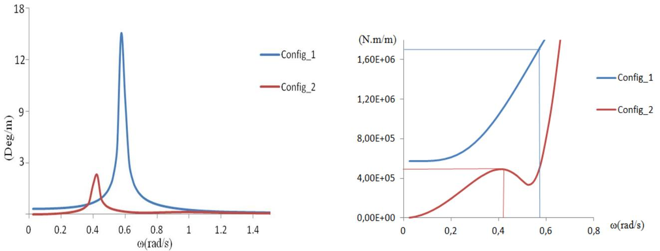
Figure 12: RAO of roll (left) and RAO of total roll excitation (right) obtained with the program DIFFRAC
