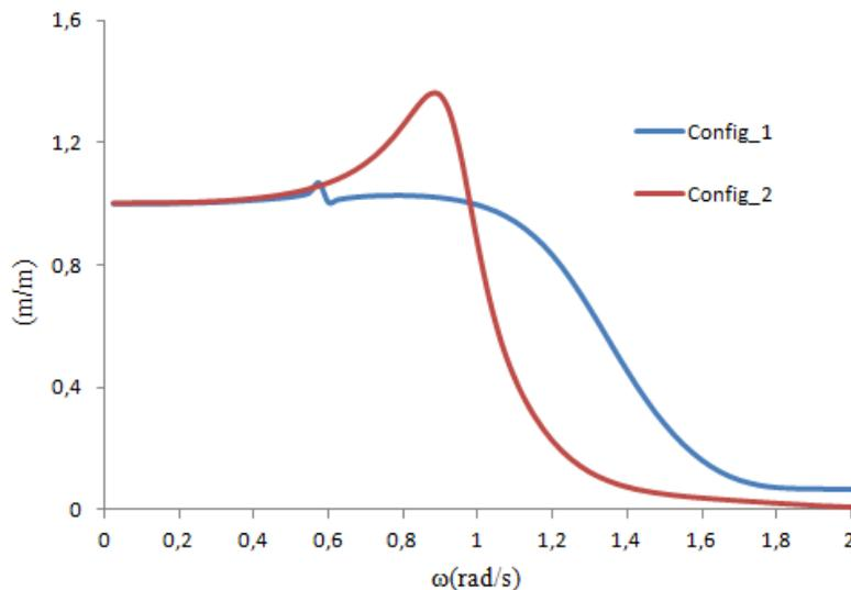
Figure 15: RAO of Heave in beam seas obtained with the program DIFFRAC
