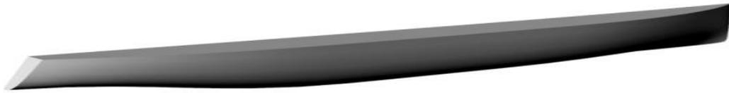
Figure 5: slender half hull of the concept yacht
