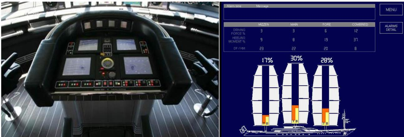
Figure 3 Maltese Falcon bridge sailing control panel (Left) and mast load display graphic (Right)
