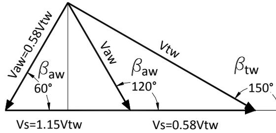
Figure 8 Wind vector triangle for downwind sailing
