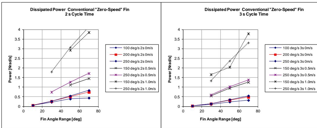
Figure 11: [Dissipated power in roll of conventional fin]
