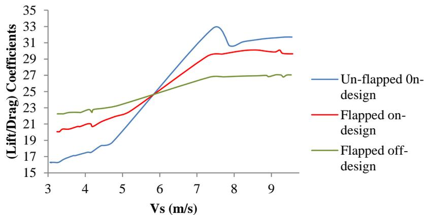
**Figure 10 Coefficients of lift/drag with respect to hull speed.**
