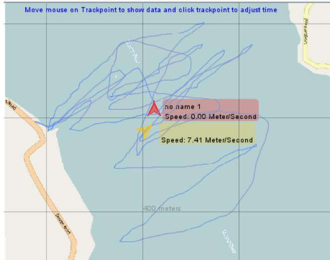
**Figure 3** GPS Action replay screen shot of un-flapped foil test session. The red arrow shows the position of the stationary wind anemometer boat, the yellow arrow and blue track line shows the instantaneous position and track of the moth fitted with the un-flapped foil.
