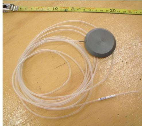
Figure 2: Pressure tap with pressure tube connected.
