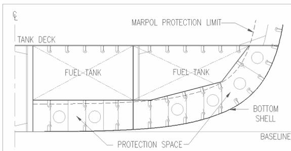
Figure 4-1: A Protected Tank Arrangement
