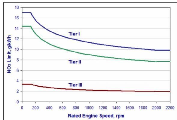
Figure 6-1: Tier I, II & III NO<sub>x</sub> Emission Limits
