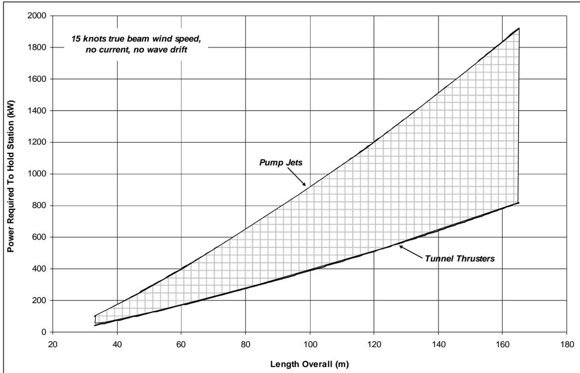
Figure 6, Power Demand To Hold Station, 15 knots True Wind Speed
