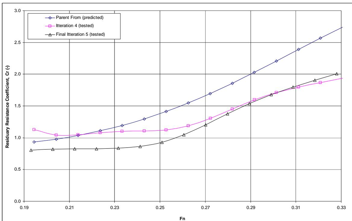
Figure 5 Final Measured Resistance Coefficients, C<sub>R</sub>
