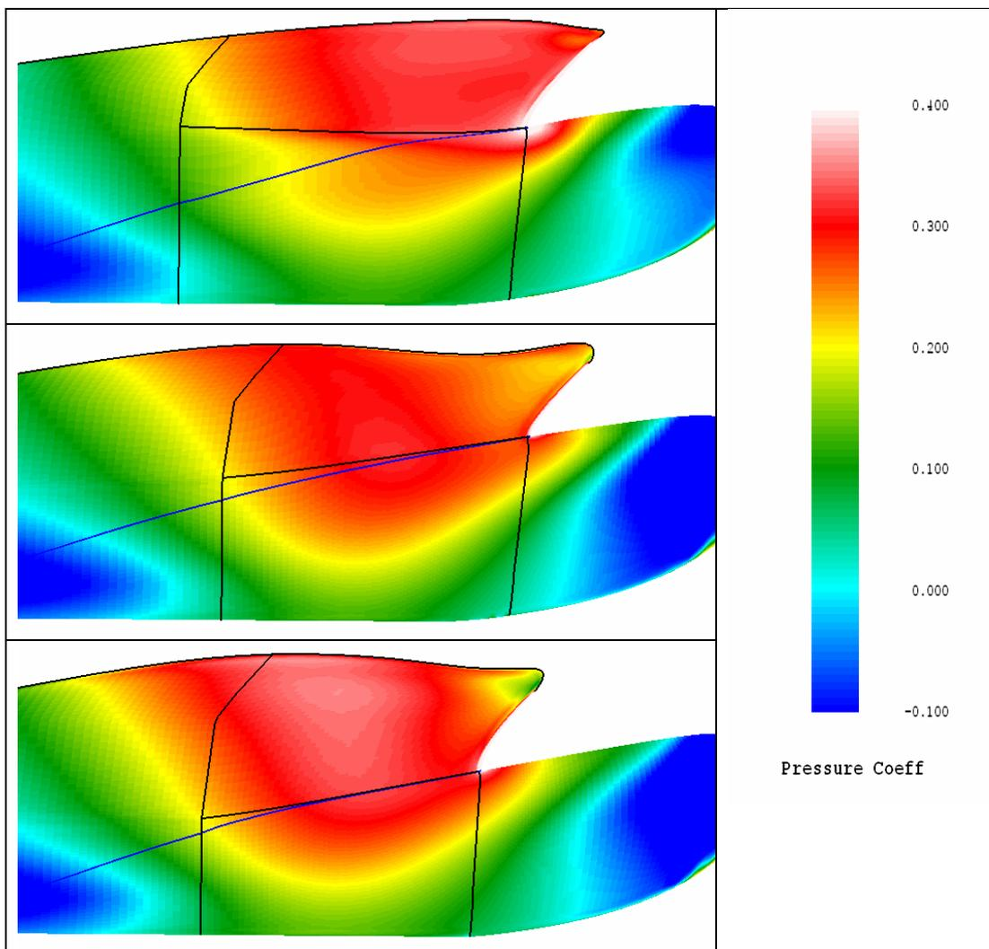
Figure 3 Pressure distribution with streamline at Vs =14 kn.
