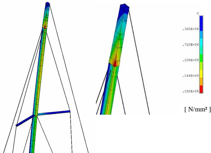
**Figure 6: Von Mises stress looking from port side**
