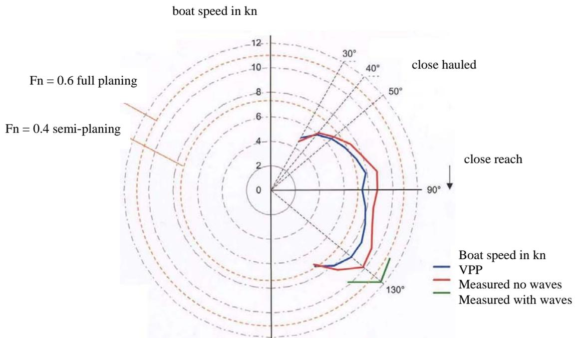
Figure 7: Polares for 12 kn (6 m/s) true wind speed
