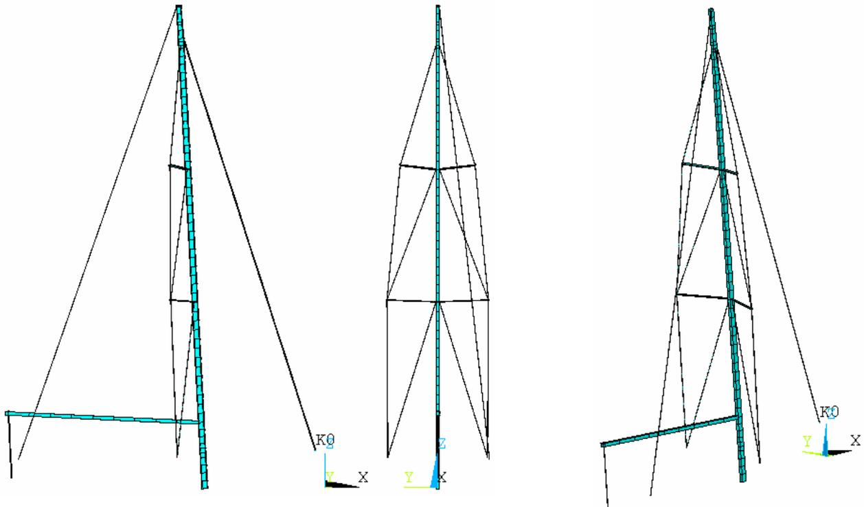
**Figure 3: Geometry of FE model, looking from starboard side, astern and 3D**
