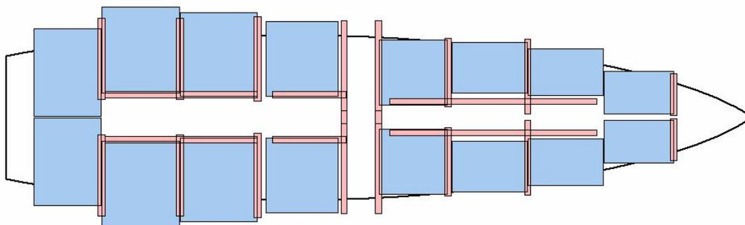
**Figure 1. HullScant output showing panel layout**
