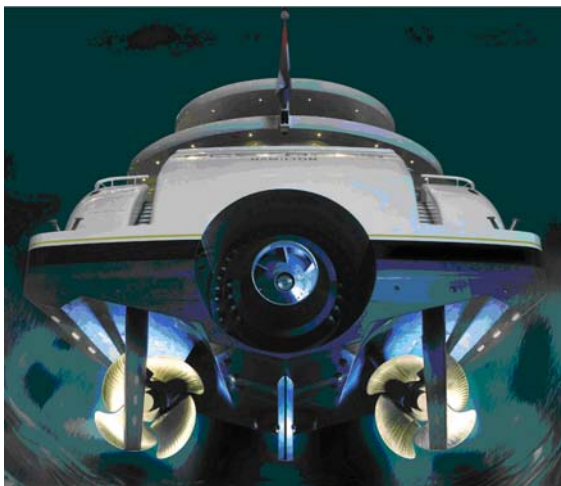
Figure 1 Hybrid propulsion with controllable pitch propellers and water jet on Ecstasea
