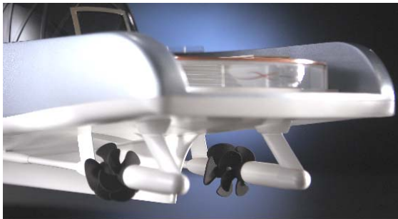
Figure 2 Hybrid propulsion with controllable pitch propeller and pod on X-stream
