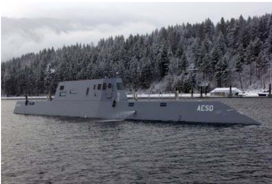
Figure 4 Advanced Electric Ship Demonstrator with submerged water jet from Rolls Royce
