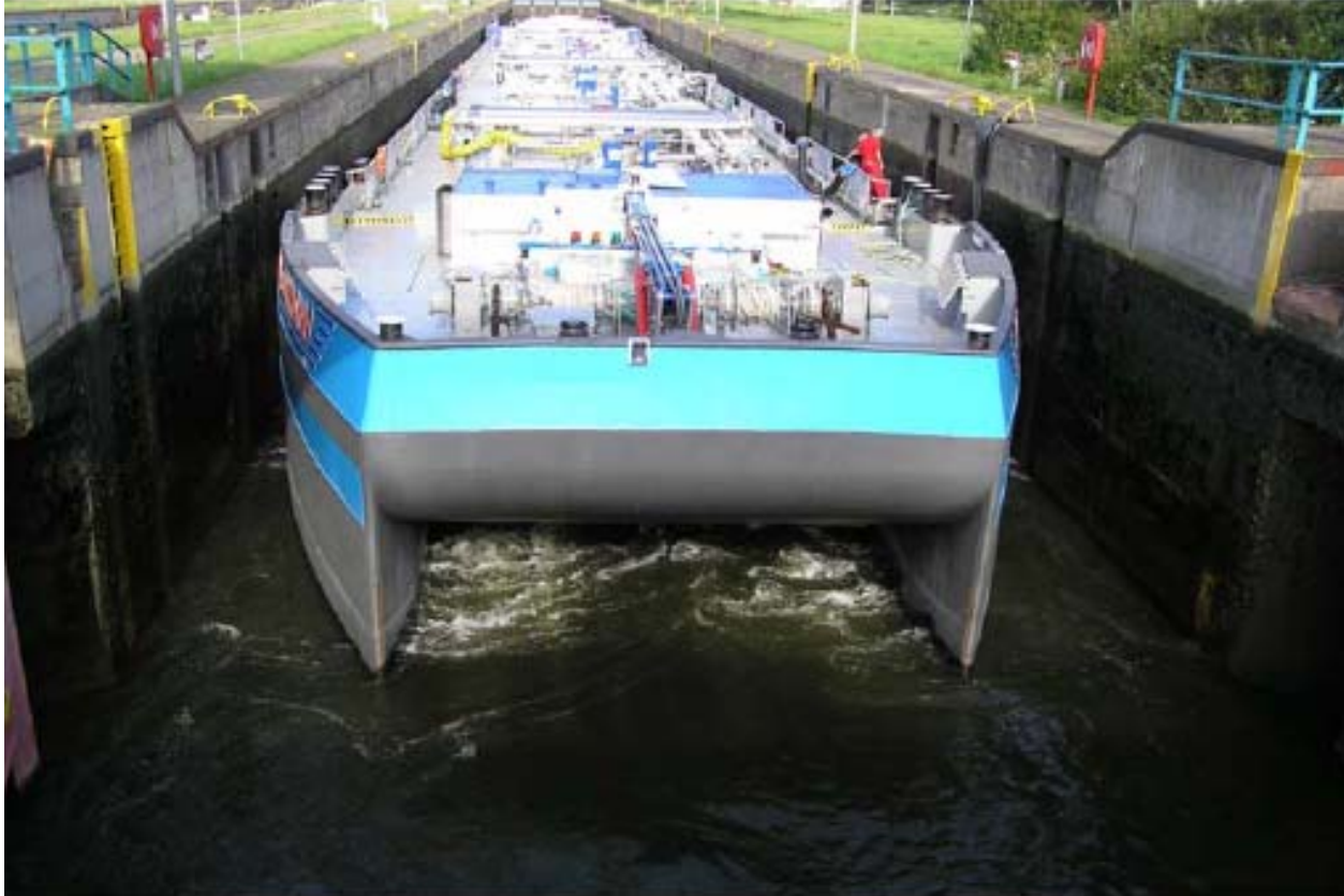
Figure 1 The Futura carrier Till-Deymann , a full-scale test ship for bubble injection, showing its typical semi twin-hull bow.
