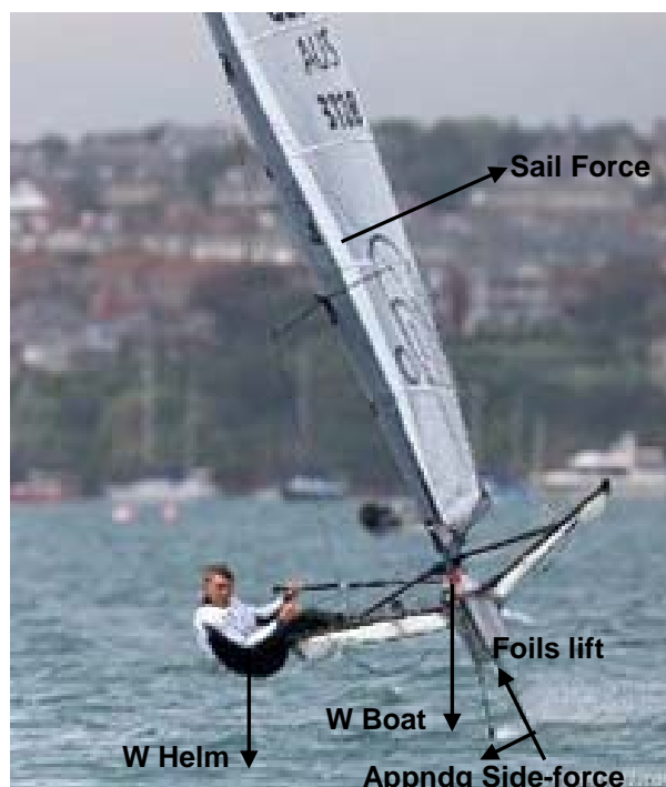
Figure 4. Demonstrating the windward heel angle and the showing the lift and weight forces. Note that drag and windage forces are not represented. Photo from [4]
