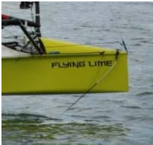
(a) Bow mounted wand sensor that tracks water surface and controls flap angle on forward hydrofoil. Photo by Hannah Kemlo.
