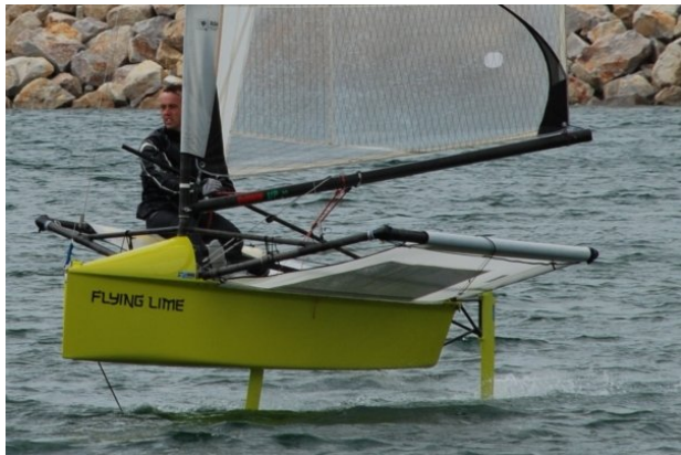
Figure 1. International moth. Showing narrow hull and wide beam overall due to ‘wings’. Appendages (daggerboard and rudder) can be seen piercing the surface and have lifting hydrofoils mounted on the submerged ends. Photo by Hannah Kemlo.
