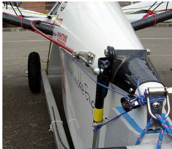
(b) The linkage between the wand sensor and the push rod which leads back to the daggerboard and mechanically controls flap angle. Photo from [5]
