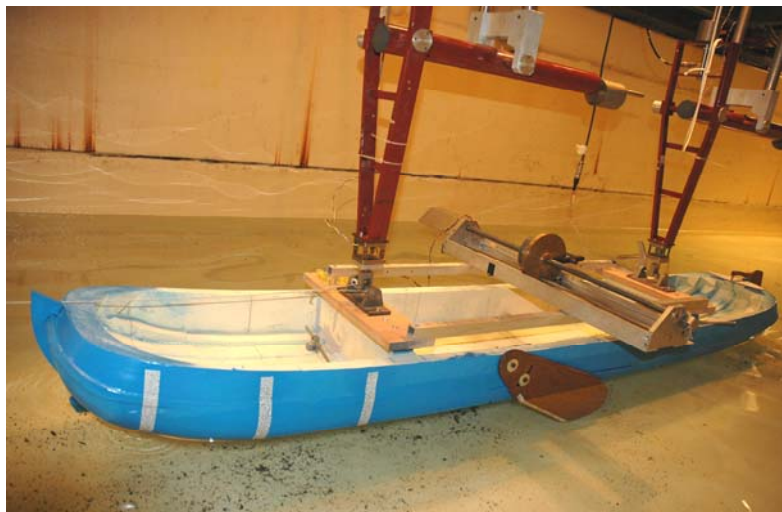
Figure 2 Test setup, three single width carborundum strips are visible near the bow
